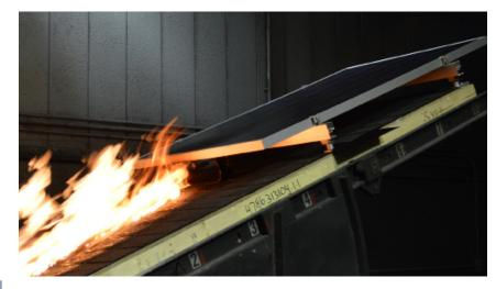
spread of flame test results. There are 15 total module types, Types 1, 2 and 3 represent differences in the module composition and Types 4 – 15 are the same module compositions as Types 1 – 3 with differing fire test performance.
