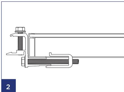
With the bolt backed out, rest the flat top side of the skirt mount onto the bottom edge of the module frame.
