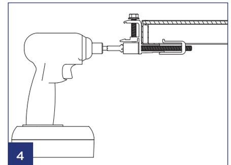
Finalize placement of skirt mount and torque hardware to 5-7 ft-lb.
