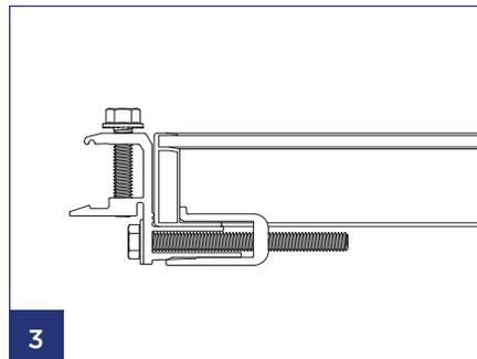
Sandwich module frame with two halves of skirt mount, ensuring that the shorter end of extrusion is facing up.
