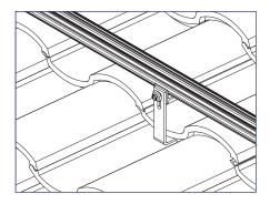
11) Install SnapNrack Ultra Rail directly to the Ultra Rail Mounting Hardware, level rails & tighten to 12 ft-lbs.
