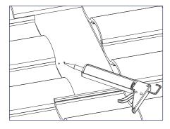
4) Apply roofing sealant to pilot holes and Tile Hook base.
