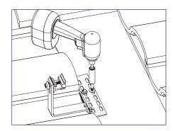
5) Attach the base with (2) 5/16" lag screws, drive lag screws for minimum 2.5" embedment into the roof framing member.
