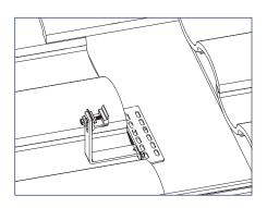
2) Align the base over the rafter so the hook can enter at the valley of a tile (all curved tile). Depending on rafter location, the hook may need to be relocated to one end of the base. Remove the nut, relocate the hook, and bolt to an end position, thread the nut back on the bolt.
