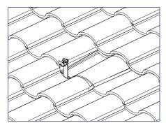
10) **OPTIONAL:** Install Tile Replacement Flashing in place of roof tile over tile hook. Flat, W, and S Tile Replacements are available.
