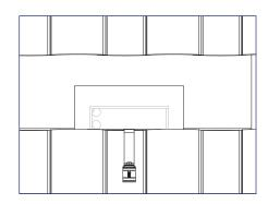
2) Peel off the backing from a 5"x13" strip of flexible flashing. Apply the strip centered laterally over the base and abutted to the Tile Hook arm. Press and roll out any creases or air bubbles with a roller to maximize contact of the flashing adhesive to 100% of the surface and base.
