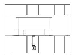
3) Peel off the backing and apply the second 4"x17" strip of flexible flashing along the top edge of the first strip with a 2" lap on either edge, then roll out any creases between the strip and the deck level surface.
