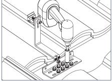
7) OPTIONAL: Drive (6) or (8) #14 Sealing Washer Wood Screws in correct mounting holes. (4) Wood screws must be used next to the hook. the remaining (2) or (4) wood screws to be installed as shown.
