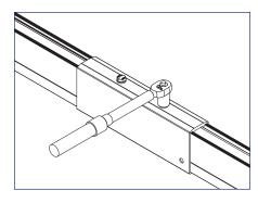
1) Slide the two rail ends into each end of the SnapNrack Ground Rail Splice, leaving a gap of no more than 1". Tighten the Splice Insert bolts to 16 ft lbs.
