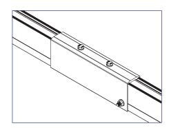
3) Insert 5/16" serrated flange grounding bolt through rail and splice, thread on serrated flange nut, and tighten to 10 ft lbs.
