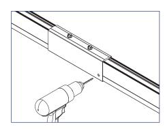
2) Drill a 5/16" hole in the Ground Rail through the existing hole in the Ground Rail Splice.
