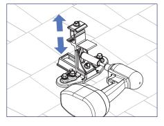
5) To set the TopSpeed™ Mount level loosen the Leveling bolt and move the clamp up or down, then tighten the Leveling bolt and torque to 16 ft-lb.
