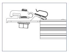
1) Slide the backplate channel of the MLPE device under the MLPE Frame Attachment Kit bolt. The MLPE mounting plate should rest against the MLPE mounting plate backstop on the MLPE Frame Attachment Kit.
