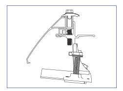
2) Column to column bonding provided by Universal Skirt and bonding clips in the Clamp assembly and/or the RL Universal Link assembly.
