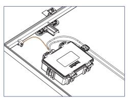
3) Run bare, solid EGC from Ground Lug R to Junction Box, bond bare EGC to stranded EGC in Junction Box. For details on installing the Junction Box reference the **Junction Box Installation Manual.**
