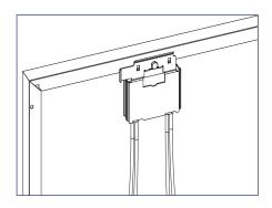
2) Install the optimizer mounting plate onto the module frame and tighten hardware to 11 ft-lbs.
