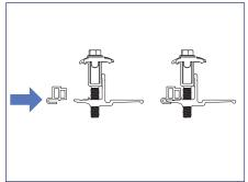
7) Universal Spacers will need to be added to Mounts and Clamps where Skirt will be installed.
