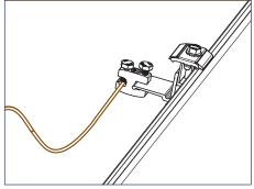
3) Each continuous array is connected to Equipment Grounding Conductor through Ground Lug (242-92202) installed on one module per array.
