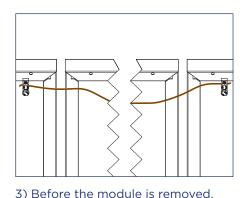
4) Service the array. With the bonding jumper installed, it is now safe to remove the module for service or maintenance.
