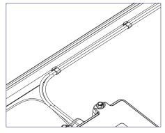
1) Use SnapNrack Smart Clip II to manage up two PV wires inside the module frame while prepping out the modules on the ground or installing modules on the roof.
