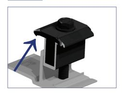
1) Row to row module bonding provided by bonding clips in Mount assembly and Clamp assembly.
