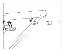
1) Ground Lug (242-92202) can be attached anywhere along the module frame or any TopSpeed™ Mount near the Junction Box. Torque module clamping bolt to 8 ft-lb.
