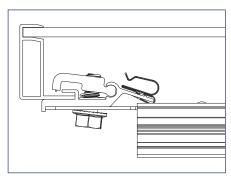
2) Position the MLPE Frame Attachment Kit on the module frame flange in a location that will not interfere with mounting system components. The module frame flange should rest against the module flange backstop on the
