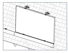
1) Rest downslope edge of module on the Mounts and/or Clamps position module so side edge is flush with marked edge of array layout or Skirt.
