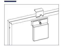
1) Locate the Enphase Frame Mount bracket clamp at a location on the module frame that will not interfere with the TopSpeed™ Mounts.
