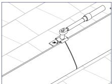
9) Use TopSpeed™ Clamps to connect multiple lengths of Array Skirt.
