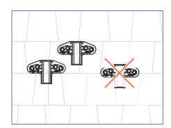
1) Install TopSpeed™ Mounts at locations drawn during the skirt layout. Mounts must be installed entirely on one course of composition.
