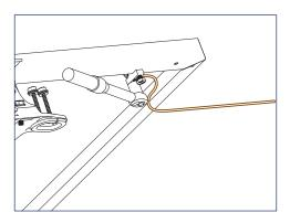
2) Run 10 - 6 AWG, solid, bare copper GEC into Ground Lug channel, torque wire clamping bolt to 8 ft-lb.
