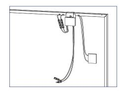
3) Connect the module leads to the input connectors on the optimizer and manage conductors with SnapNrack Smart Clips.
