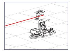
6) Pull string line tight from one corner mount to opposite corner mount to align and level all TopSpeed™ Mounts between the end mounts.
