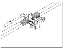
3) Tighten 1/2" clamping bolt to 16 ft-lb. Only two Mounts are required per module on one side.
