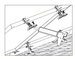
4) Lift the upslope edge of the module and fill the SpeedSeal™ reservoir with roofing sealant.
