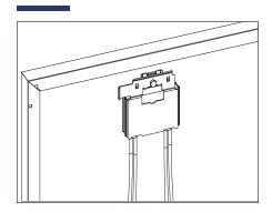
1) Locate the SolarEdge optimizer with Frame-Mounted Module Add-On at a location on the module frame that will not interfere with the TopSpeed™ Mounts.
