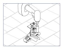
3) Attach TopSpeed™ Mount to roof using the (4) SnapNrack #14 Wood Screws with 1/2" hex head that are captured in the Mount.
