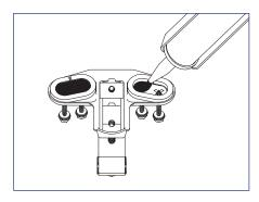
2) Fill both cavities on bottom of TopSpeed™ Mount created by SpeedSeal™ gasket with roof sealant to ensure a watertight seal.
