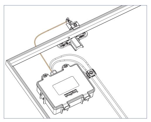
4) Optionally; Install Ground Lug on the Mount Landing Pad at the top of the array. Run bare copper between ground lug and Junction Box.
