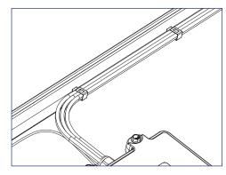
2) Use SnapNrack Smart Clip XL to manage larger bundles of PV wire; up to 6 PV wires per clip
