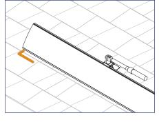
8) Install Universal Skirt by holding the skirt in Mount, sliding Skirt to align with array layout marks, and clamping skirt into mount.
