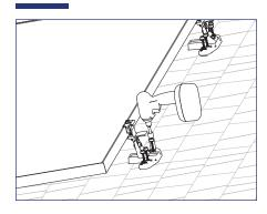
5) Lower the module to the roof and drive the (4) pre installed Snapnrack #14 Wood Screws with 1/2" hex head into the roof sheathing.
