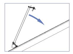
2) Lower upslope edge of module while simultaneously applying slight pressure to seat module into Mounts and/or Clamps.
