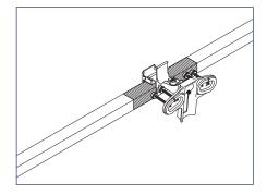
2) Position TopSpeed™ Mount clamp on the module frame within the module manufacturers required clamping zone.
