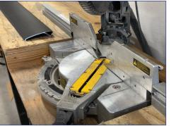
For an inside and outside miter joint on opposing ends, take a measurement of the length of the array edge or panel length and add  $\frac{3}{4}$ ".
