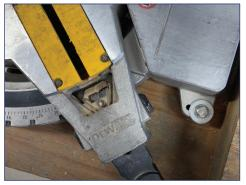
For a single inside miter joint, measure the array or panel length and cut to the exact length. Adjust the saw to the 45° angle and cut the skirt with the flat side seated flush against the fence.
