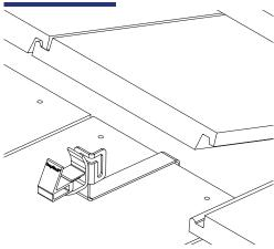
1) Lift tile in course above Universal Conduit Mount, Tile location, slide conduit support underneath the lifted tile and hook it over tile below so bent end of hook rests against tile, then lower tile onto the hook. For curved "W" or "S" tile profiles, the Universal Conduit Mount, Tile should be located at the **hightest** point in the tile.
