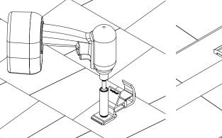
3) Place conduit into the opening of the conduit clamp, adjust conduit to desired position
