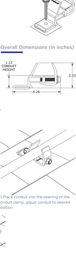
4) With a 1/2" socket or driver, tighten conduit clamp hardware to torque listed under General Information
