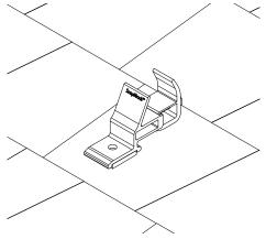
1) Remove protective liner from the butyl and place the Universal Conduit Mount, Simple at desired location on the roof.
