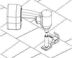
2) With a 1/2" socket or driver, drive the #14 wood screw into the roof decking. Tighten until the sealing washer is compressed.
