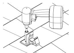
2) With a 1/2" socket or driver, drive the #14 wood screw into the roof decking. Tighten until the sealing washer is compressed.
