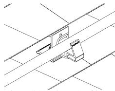
3) Place conduit into the opening of the conduit clamp and adjust height to desired position
