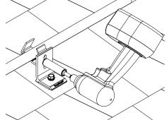
4) With a 1/2" socket or driver, tighten conduit clamp to torque listed under General Information
