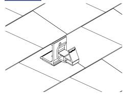
1) Remove protective liner from the butyl and place the Universal Conduit Mount, Leveling at desired location on the roof.
